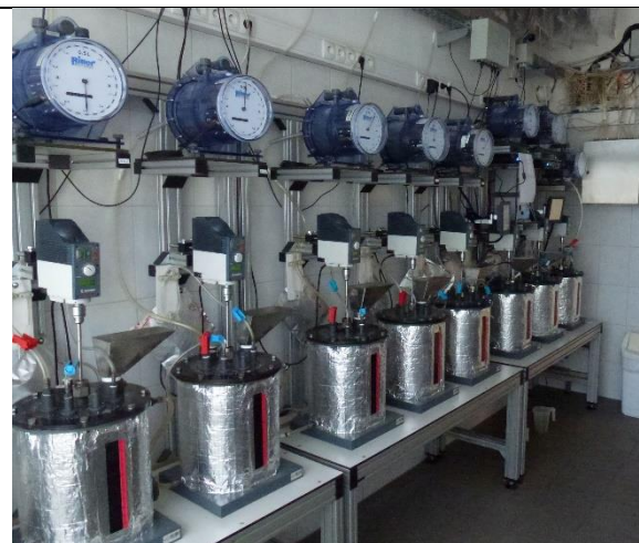
Figure 2: Lab reactors (CSTR) with 15 L working volume
