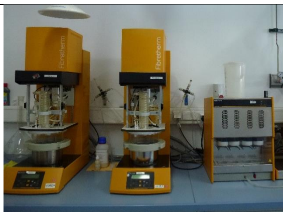
Figure 5: system for automated disintegration to determine cellulose, hemicellulose and lignin (crude fiber, XF)
