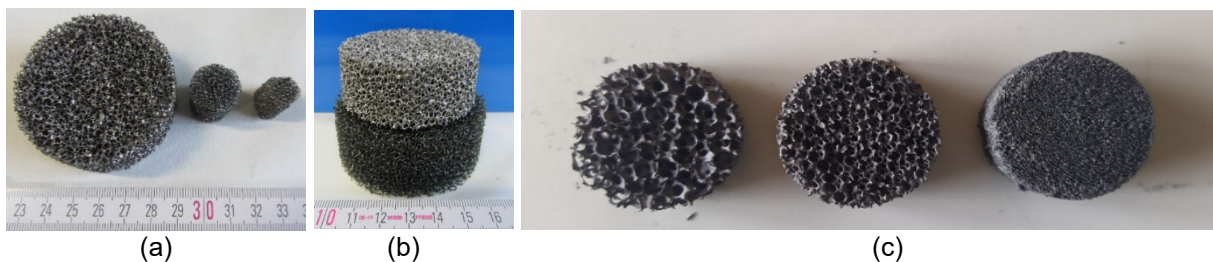
Figure 2. (a) In-house manufactured 30 ppi \text{Ca}_{0.90}\text{Sr}_{0.10}\text{MnO}_3 foams of Ø 65, Ø 20 and Ø 10 mm. (b) Comparison of Ø 65 mm sintered \text{Ca}_{0.90}\text{Sr}_{0.10}\text{MnO}_3 foam (on top) to the Ø 80 mm PU foam template used for its preparation, to delineate shrinkage due to sintering. (c) \text{CaMnO}_3 foams of Ø 20 mm of 20, 30 and 60 ppi.
