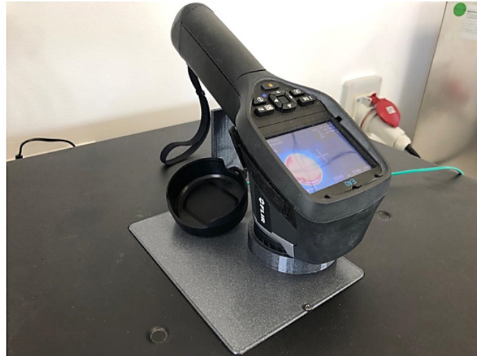
Figure 2. IR camera allocated on the microwave oven, looking at its interior from above.
