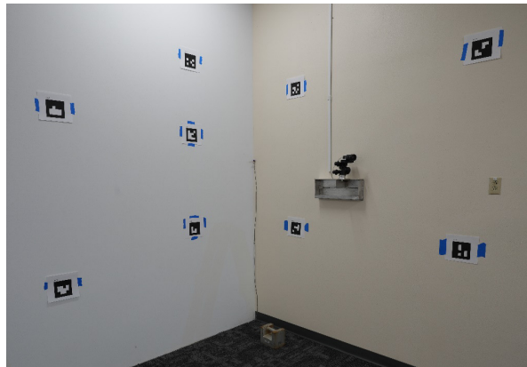
Figure 4. Example of photogrammetric component calibration measurement setup.
