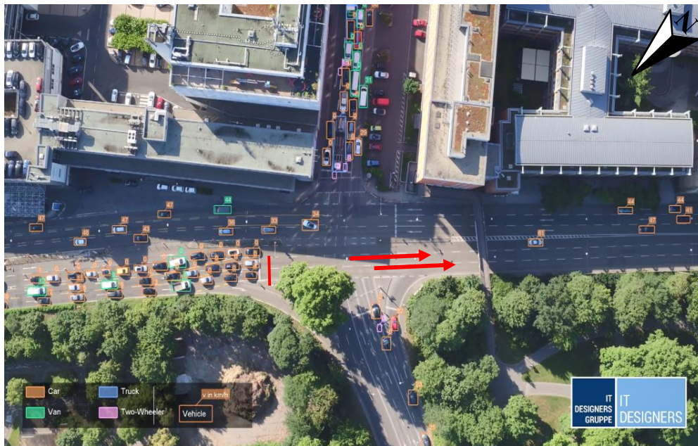
Figure 3: Drone recording of the signalized junction with bounding boxes and vehicle types
