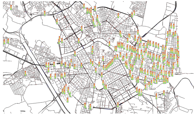
Figure 1: A part of the Traffic Lights definition in Valencia's network.
