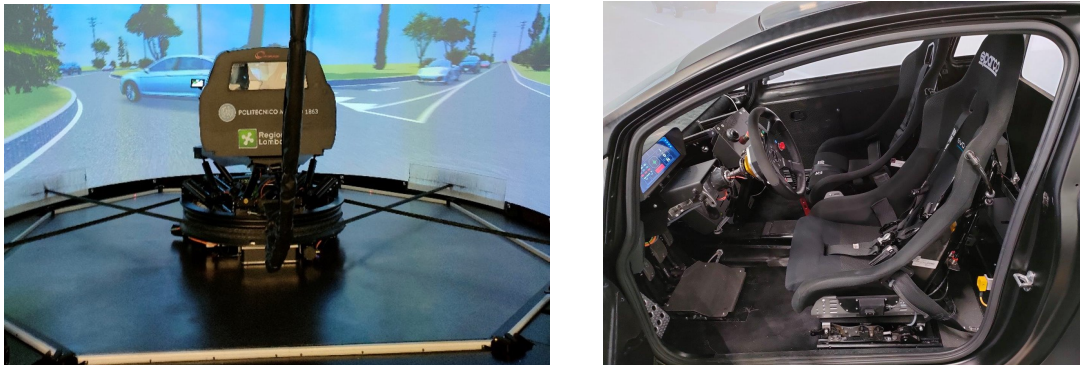
Figure 1. Driving simulator DIM400 at Politecnico di Milano inside the DRISMI lab ( www.drismi.polimi.it ). On the right, detail of the cockpit interior.
