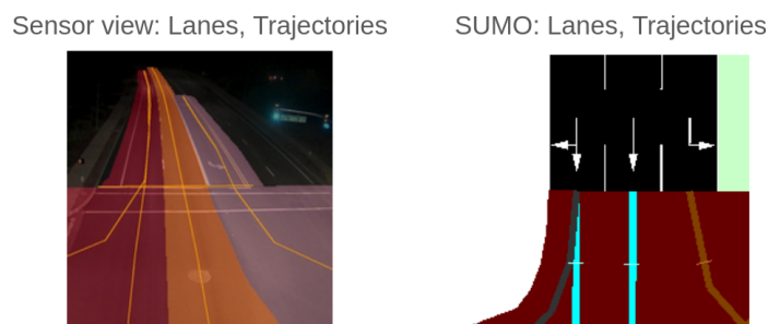
Figure 4. SUMO network approach edge and connections generated from NoTraffic™ cloud data.
