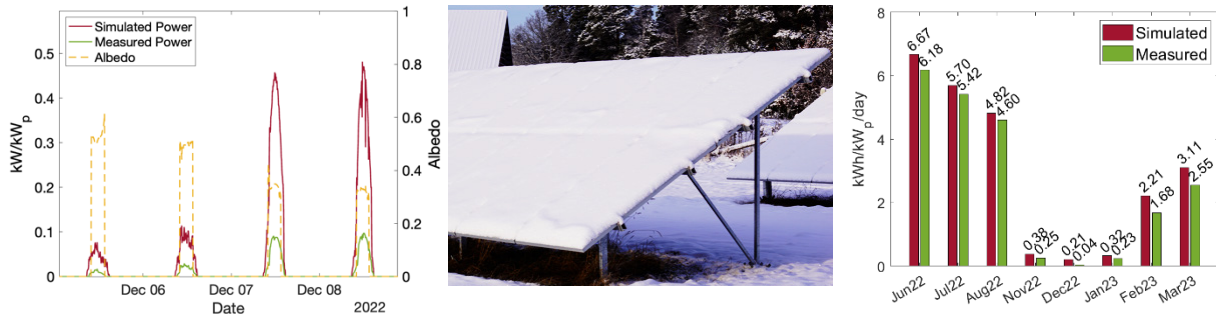
Figure 4. Left: Comparison between simulated and real measured AC power during a period with snowfall using 5-min data for the GM system in Västerås, Sweden. Center: Photograph of the GM system in Västerås covered with snow. Right: Comparison of simulated and measured average daily specific yield per month for the GM system. Note that certain months may be omitted or may not include data for all days due to data quality issues or missing data.
