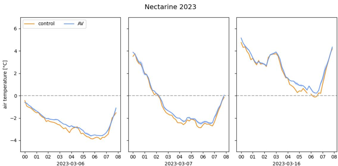
**Figure 4.** Air temperature at night nearby control and AV nectarines during the 2023 bloom period. Each curve is the mean value of two thermo-hygrometers for control and four thermo-hygrometers for AV trees.
