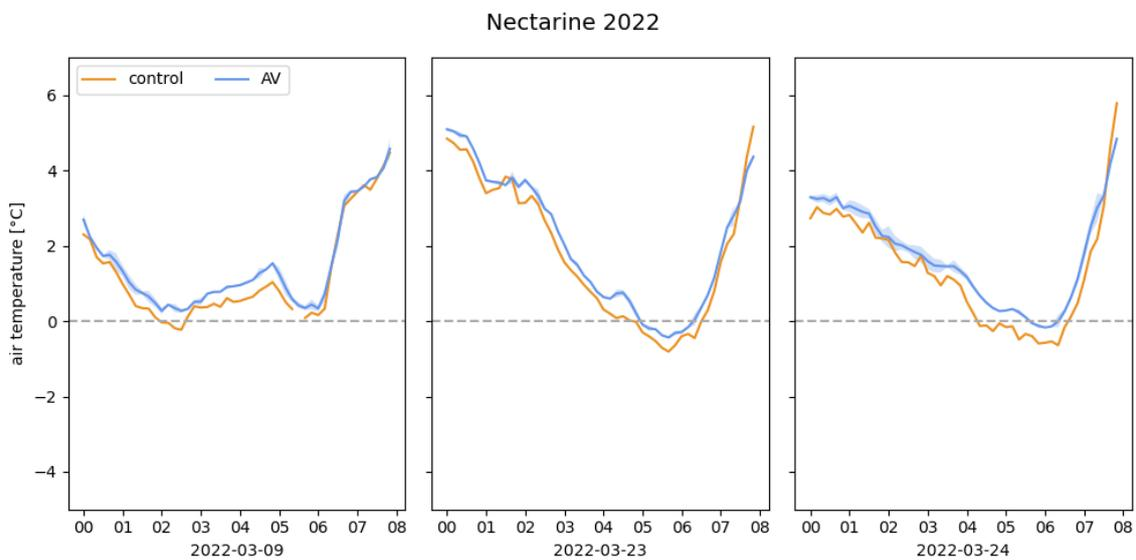
**Figure 3.** Air temperature at night nearby control and AV nectarines during the 2022 bloom period. Each curve is the mean value of two thermo-hygrometers for control and four thermo-hygrometers for AV trees. On March 9, anti-frost candles were used in the orchard explaining the increase in temperatures at the middle of the night (ca. 02:30).
