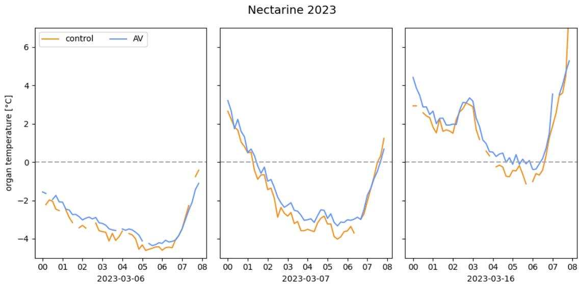
**Figure 5.** Estimation of organ air temperature using a frost sensor that mimic organ temperature nearby control and AV nectarine trees during the 2023 bloom period.
