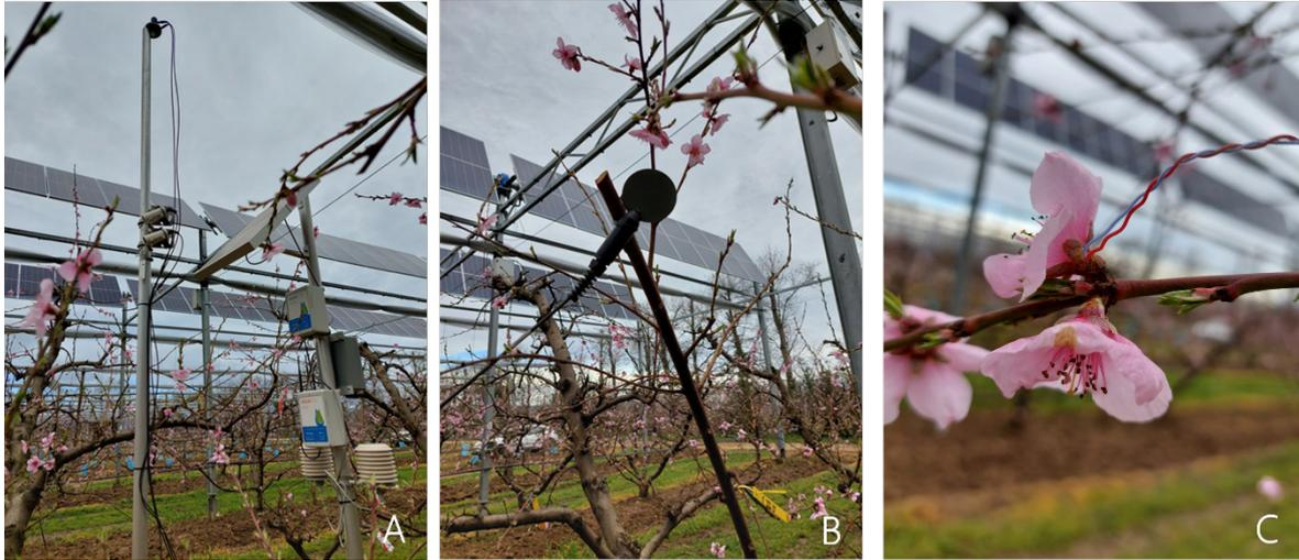
**Figure 2.** Different methods used to identify frost events in nectarine: thermo-hygrometers to measure air temperature nearby the trees (A), frost sensors to mimic organ temperature (B), and thermocouples inside flower buds (C).
