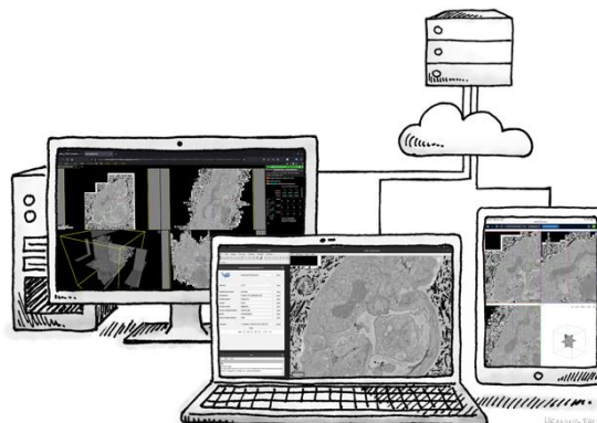
Figure 3. Several visualization tools already support OME-Zarr, including Fiji/Bigdata-viewer/MoBIE [16] on the desktop, webKnossos [17] and Neuroglancer [18] on the web. With OME-Zarr, a selection of software tools and devices can access the same datasets from centralized storage. "Multiple clients" by Henning Falk, ©2022 NumFOCUS, is used under a CC BY 4.0 license. [2]
